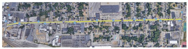
In collaboration with The City of Rochester, the project's scope of work includes a full reconstruction of East Main Street - from Goodman Street to Culver Road (yellow line). The relocation of approximately one and a quarter mile of electrical circuits is critical to the success of the project, requiring reconnection to existing routes through two miles of new underground duct banks.
